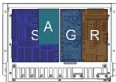
Interface circuit arrangement in NQE-1143 Junction Box
